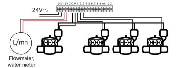
Connect your + S - input to a water meter equipped with a flow sensor as shown above. Use dry contact flow sensors or equivalent.
