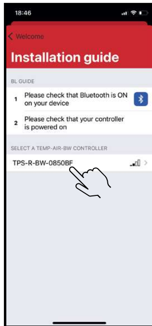
Select the required Tempus Air BW to be installed from the list of the available modules
