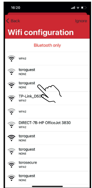
Select the WiFi network access to which you want to connect your Tempus Air BW by clicking on the corresponding line or «Ignore» if your Tempus Air BW has already been assigned to a WiFi network.
