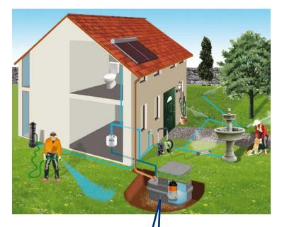
To operate correctly avoiding frequent restarts and for greater energy saving it is necessary to install the 1 SF tank (or a similar tank with a minimum capacity of 1 litre) with an initial load of 1.2 bar Maximum delivery height 1SF NT 10 m White minimum 500 mm Ц Í 2 δ ğ DEELECTRONES (CONTROL HE HERE 35 mm 🛙 minimum 300 mm
